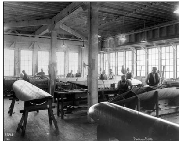
George Pocock (2nd from right), his brother Dick (far right), and their Boeing co-workers craft pontoons for the Model C, Boeing's second design. (1918 photo courtesy of Boeing Archives.)
